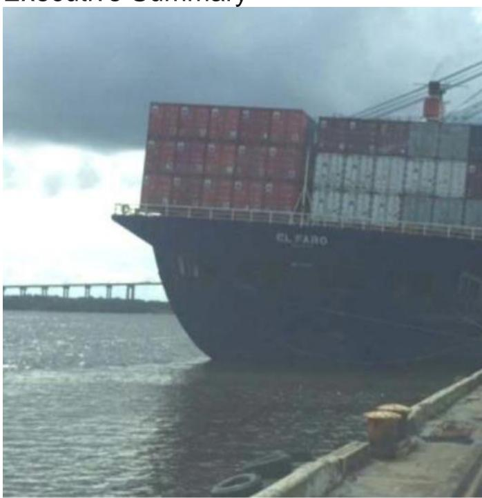
The final photograph taken of the El Faro by TMPR Terminal Manager on September 29, 2015, showing starboard list of approximately 4 degrees during loading operations prior to the final voyage. Credit: U.S. Coast Guard
